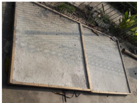
Figure 2. Concrete Panel Specimens.
