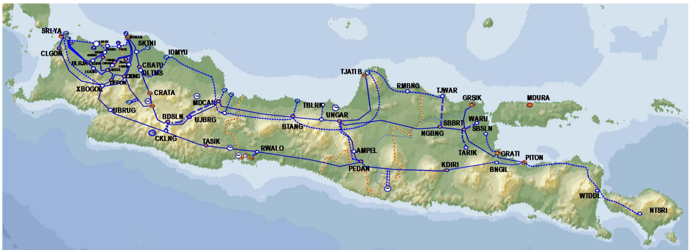
Fig. 2. Jawa-Madura-Bali 500 kV single line diagram [3]
