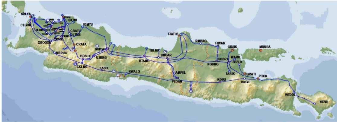
Fig. 2. Jawa-Madura-Bali 500 kV single line diagram [3]
