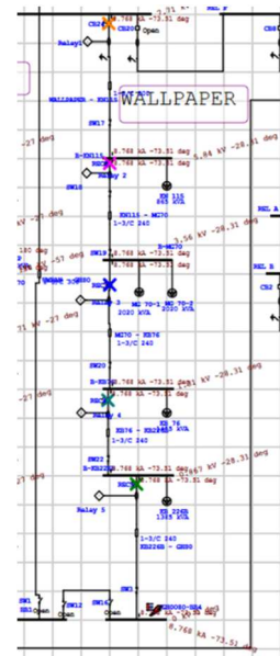
Figure 7 Protective Coordination on Wallpaper Feeder
