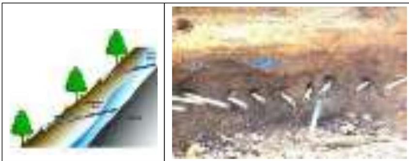
**Gambar 9.25.** : Sistem drainase air tanah (*subsurface drainage*)
